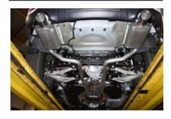
6. With both mufflers in place align both parts so they match each other and are centered in the exhaust outlets. You may need to use something like a rag to hold the tips in place while the clamps are being tightened.
